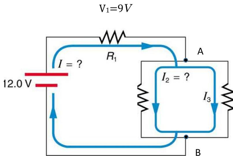
$$V_2 = V_3 = 3V \text{ (from A to B)}$$
