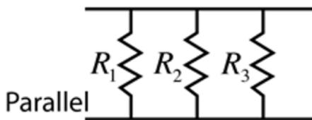
$$\frac{1}{R_{equivalent}} = \frac{1}{R_1} + \frac{1}{R_2} + \frac{1}{R_3} + \dots$$
