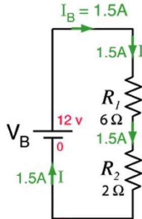
**No split** in this series circuit means the **current** always remains at **1.5A everywhere** in the circuit.
