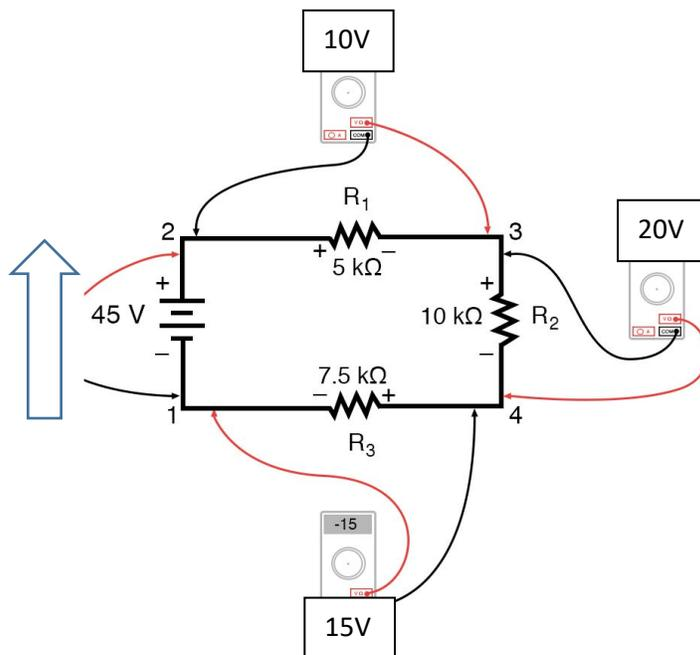
$$45\text{Volts (supplied)} = V_1 + V_2 + V_3 \text{ (all voltage lost)}$$
