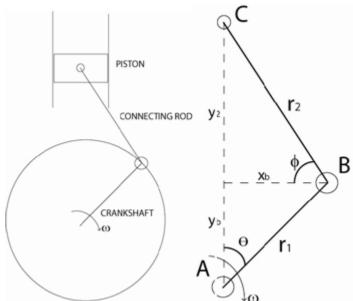
The <u>rate</u> at which the **piston** moves down is <u>related</u> to the <u>rate</u> at which the **crankshaft** turns
